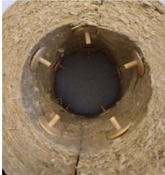
Figure 4 - ESSGE NCS spacer buttons in two rows with 5 pcs each and a C-C of 100mm
